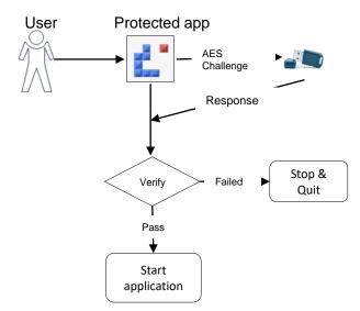
Moway support HMAC-SHA1/SHA256, AES, symmetric cryptographic to deploy Challenge/ Response authentication process
